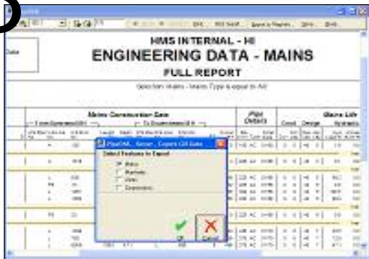
A report showing all 'AC' pipes is generated in PipePAK . Export to MapInfo is chosen from the toolbar, 'Mains' is selected and the OK button clicked.
