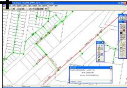
Focus is automatically switched to MapInfo. All 'AC' Mains are coloured on the map in a user-definable colour and style.
